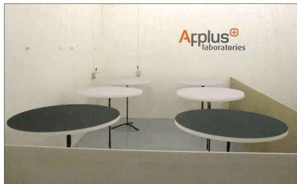
Images 5 and 6 Test specimen installation into the reverberation room
