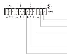
WPaVOL-SR RJ45 pin 6 (+12VDC/+10VDC) WPaVOL-SR RJ45 pin 2 (Remote VOL.) WPaVOL-SR RJ45 pin 1, 3 or 7 (GND)
