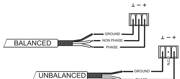
Signal output connectors are 3 position screw terminal block. The wiring is:
