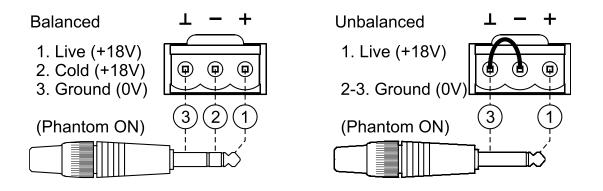
*Note:* Microphones must be low impedance (200 to  $600\Omega$ ) and monophonic.
