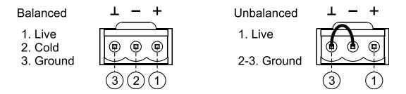
In order to use a unbalanced output, you need to short pin 2 and pin 3, as indicated in the previous diagram. Otherwise, the output signal won't have the right level and quality.
