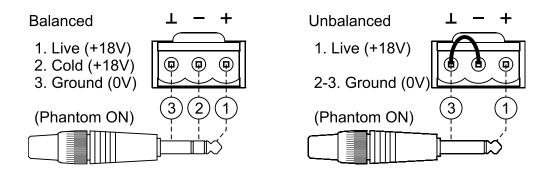
*Remark:* Microphones must be low impedance (200 to  $600\Omega$ ) and monophonic.
