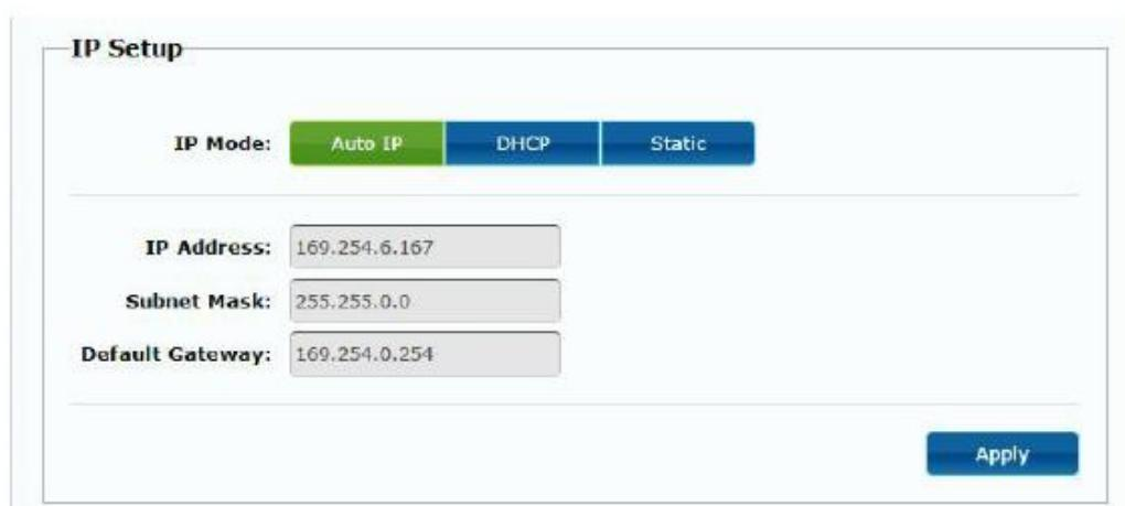
This screenshot shows the IP Setup section of the configuration interface, where the "Auto IP" mode is selected. It includes fields for IP Address (169.254.6.167), Subnet Mask (255.255.0.0), and Default Gateway (169.254.0.254), along with an "Apply" button at the bottom right.
