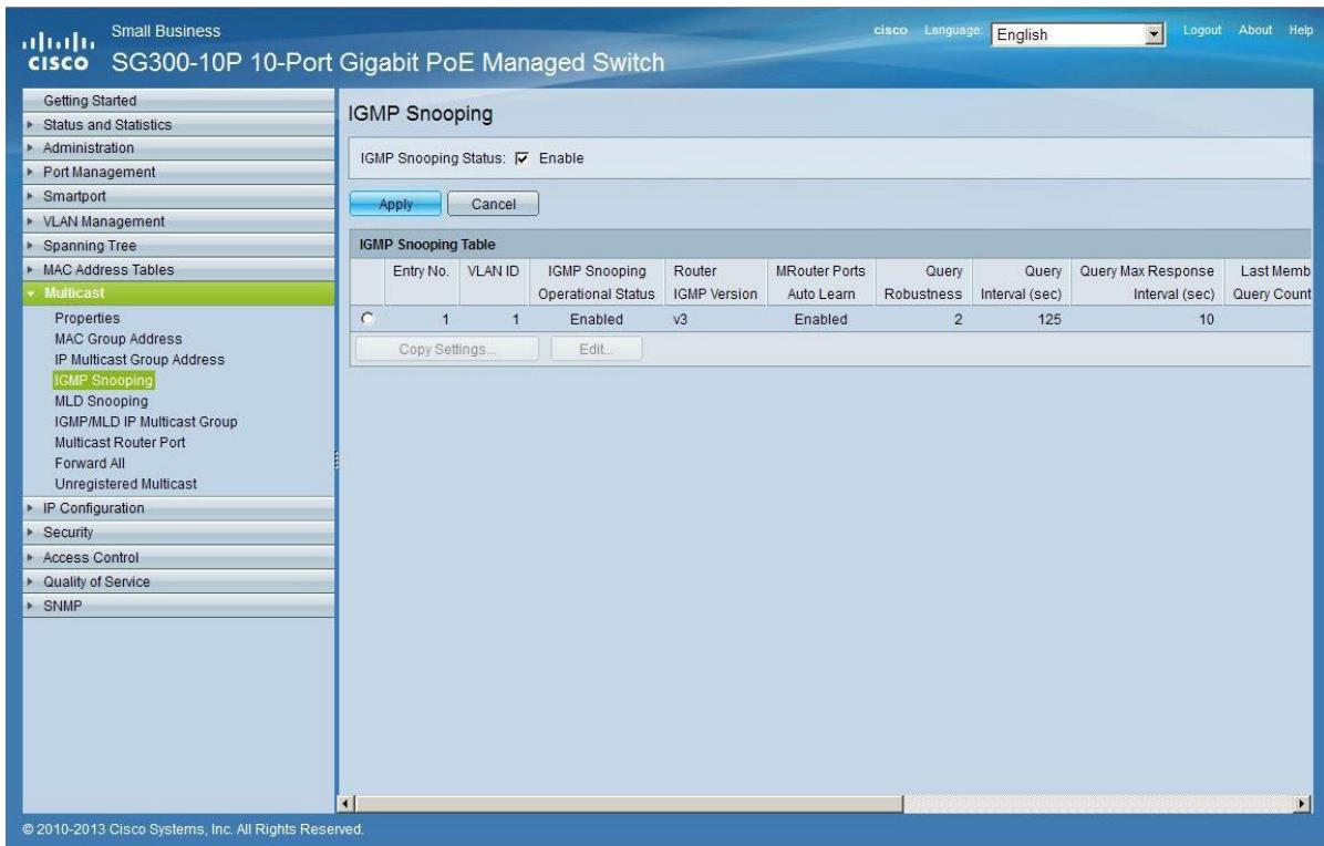
The screenshot shows the Cisco SG300-10P web interface. The left sidebar has a 'Multicast' section selected, with 'IGMP Snooping' highlighted. The main panel displays the 'IGMP Snooping' configuration. The 'IGMP Snooping Status' checkbox is checked and labeled 'Enable'. Below it is a table titled 'IGMP Snooping Table' with one row. The row contains the following values:
