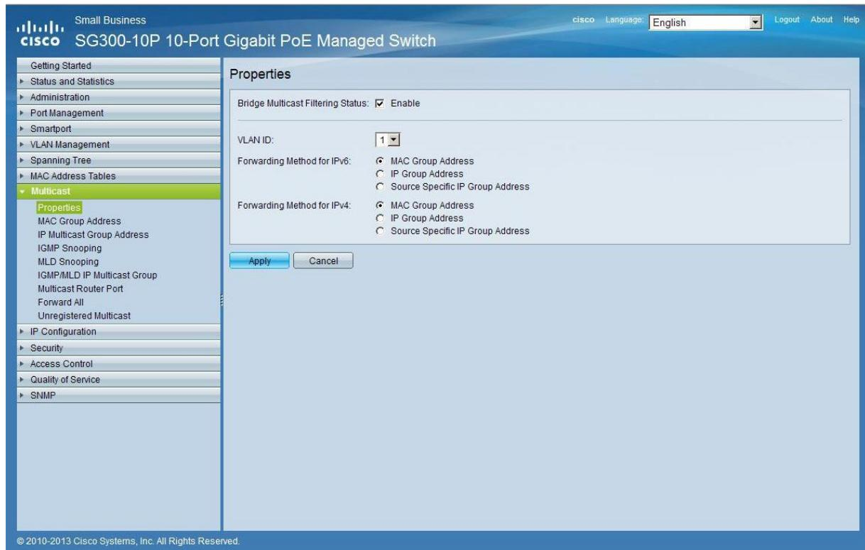
2. Select **Multicast → IGMP Snooping**. Enable the **IGMP Snooping Status** by activating the related selection box and clicking on **Apply**.
