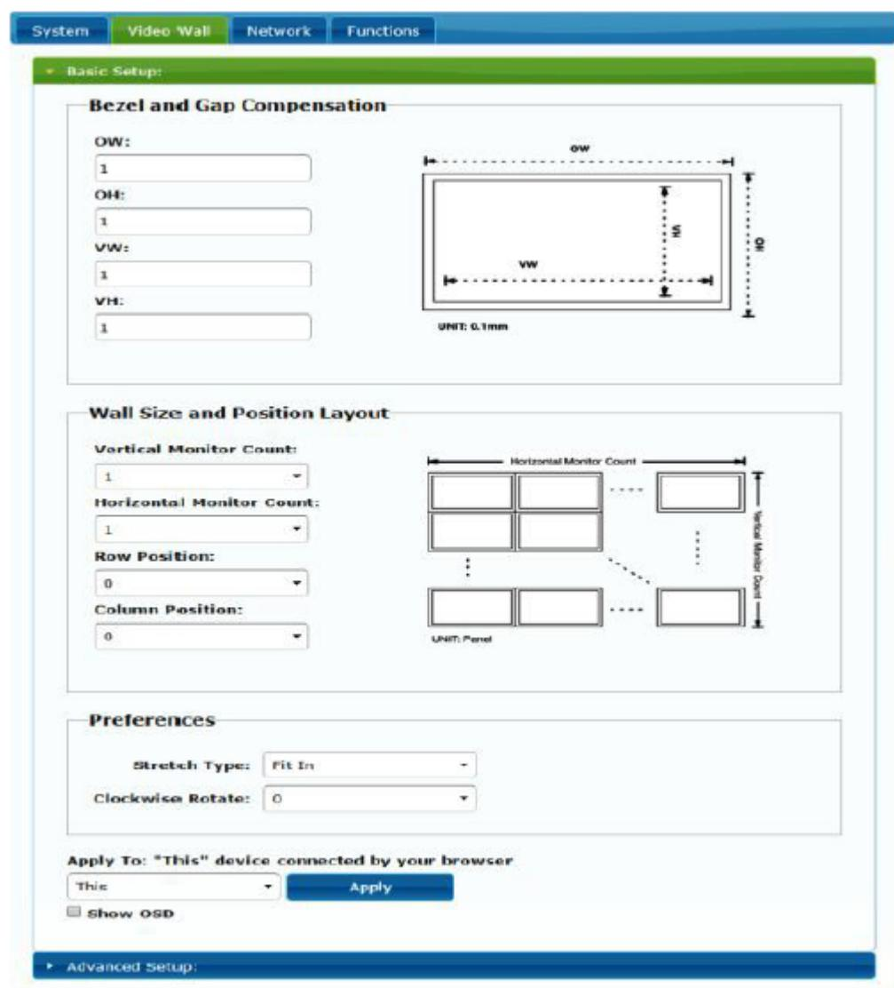
The screenshot shows the 'Basic Setup' configuration interface for a video wall. The top navigation bar includes tabs for System, Video Wall (selected), Network, and Functions. The main content area is divided into several sections:
