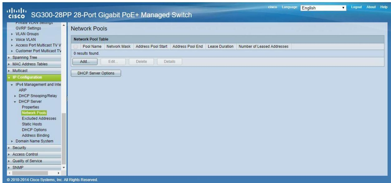
3. Set the **Pool Name**, the **Network Mask** (255.255.255.0), the **Address Pool Start** (192.168.1.10), and the **Address Pool End** (192.168.1.100). Verify that you allocate enough IP addresses for all Transmitters and Receivers present on the network.
