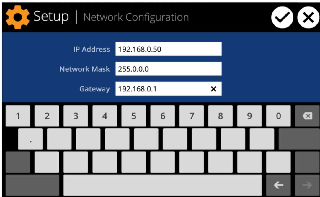
This menu allows modifying the network connection parameters of the WPNETTOUCH unit: IP address, network mask and gateway.
