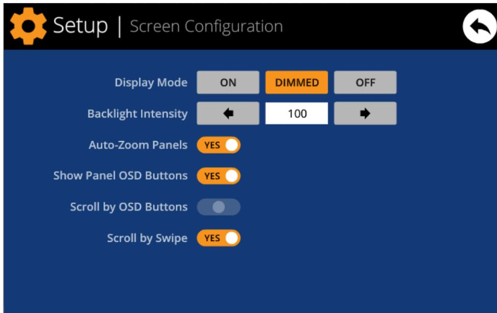
This menu allows setting different parameters affecting the displayed items and controls on the screen of the unit:
