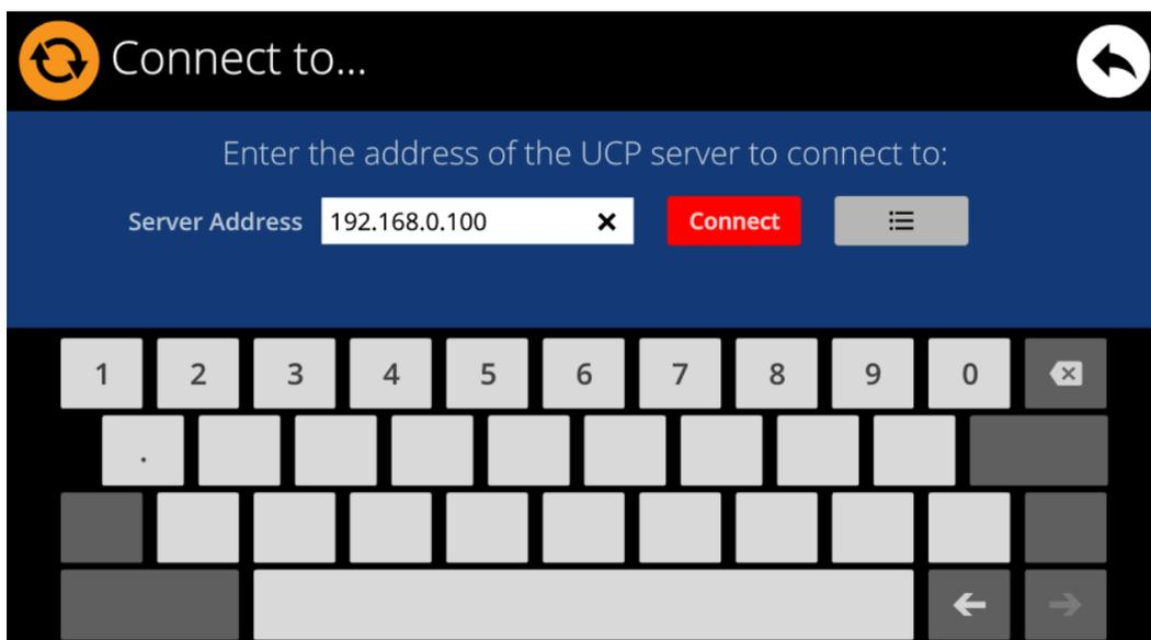
This page allows deciding the UCP server the unit will connect to as a client. The UCP server may be a computer, a MIMO4040DN matrix (yes, it has an embedded UCP server in its engine!) another WPNETTOUCH / WPmSCREEN unit or even the same WPNETTOUCH unit. In any case, the UCP server shall host and run an EclerNet Manager project that includes a series of UCPs which can be remotely managed by any UCP client.
