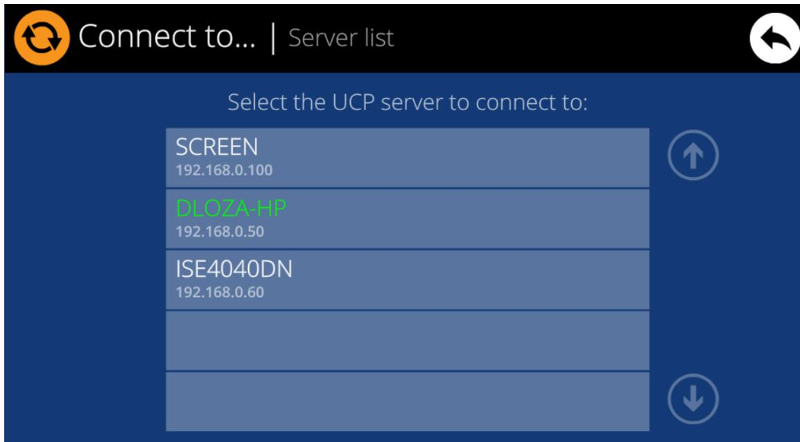
**Note:** in the list of detected server devices, the name of the WPNETTOUCH unit under control will appear in green (the one matching with the Local IP Address)
