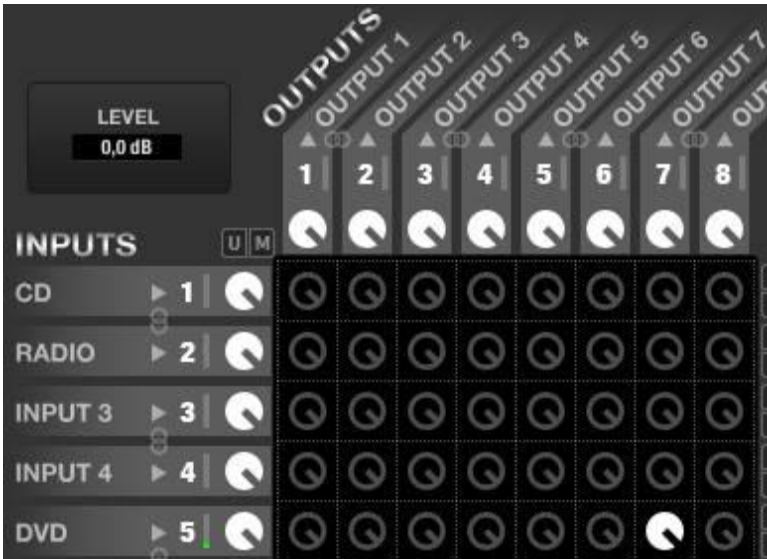
Input 5 (DVD) selected as sound source for output 7. In X-Focus mode the volume control operates the crossing point between input 5 and output 7 (filled in white in the picture)
