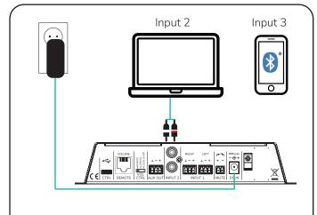
Connect the transmitter DC adapter to the electrical outlet and use one of the 3 available audio inputs to connect the music source
