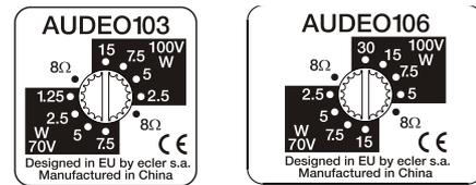
The four 100 V power line switch positions allow you to set the maximum power that will be used by each unit. Thus, in areas where a low sound level is required, the lower positions are used (5 or 7.5 W for the AUDEO106 / 2.5 or 5 W for the AUDEO103), while in areas in which a higher level is required, the higher positions are used (15 or 30 W for the AUDEO106 / 7.5 or 15 W for the AUDEO103).
