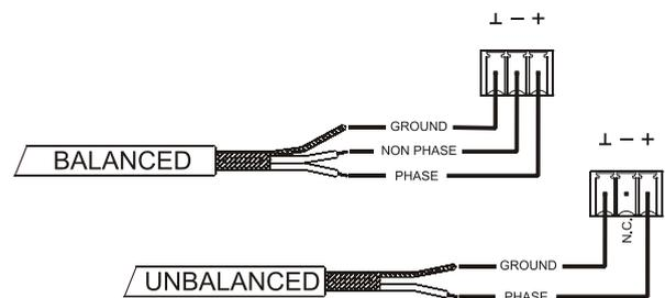
For unbalanced connection, don't connect the terminal -.
