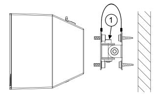
**NOTE:** As a general safety rule, remember to put the runner in place and also that the screw marked "1" should be placed at the upper part of the support, so that if it becomes loose, it will not fall.
