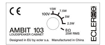
The AMBIT103 has 4 power handling levels for the 100V line. Depending on the intended use, the speaker output can be attenuated more or less. In the zones where sound intensity should be low, place the switch in the 2,5W or 5W position. If sound intensity should be high, place the switch at 7,5 or 15W.
