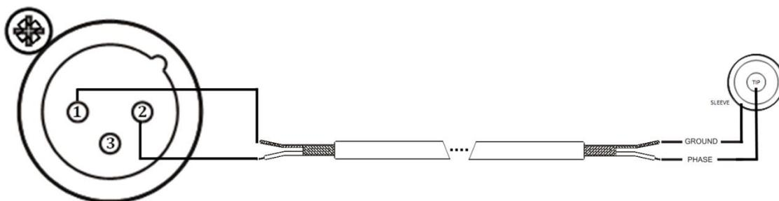
2. Connection from balanced output to unbalanced input
