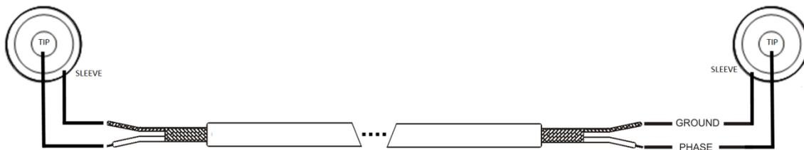
3. Connection from unbalanced output to unbalanced input
