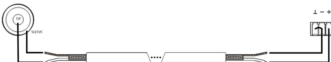
4. Connection of unbalanced output to balanced input
