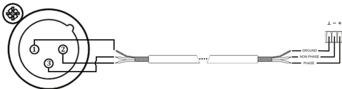
1. Connection from balanced output to balanced input
