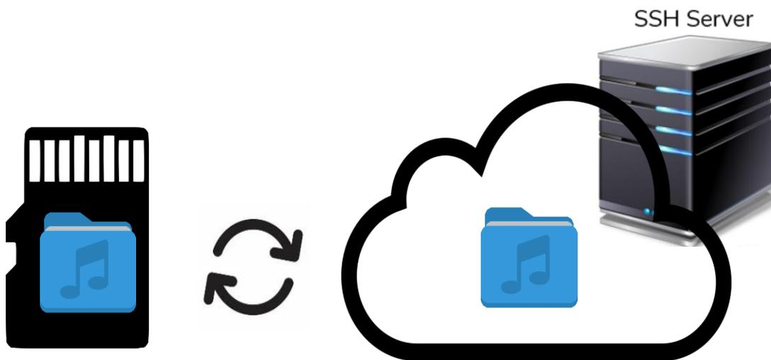
Figure 43: syncing folders with Store and Forward (rsync)
