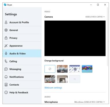
Now your Skype<sup>©</sup> camera will be the device connected to the VEO-CAP4U HDMI input and your microphone will be the device connected to the VEO-CAP4U Line In.
