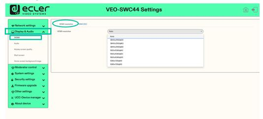
If the display only supports FULL HD, the 4K resolution will not be displayed on the resolution list.
