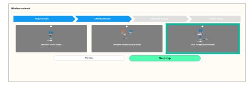
In this configuration the built-in WiFi access point of VEO-SWC44 is disabled.
