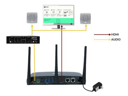
VEO-SWC44TH and VEO-SWC44TU can transmit audio to the VEO-SWC44 base unit when the audio output of the source device is selected.
