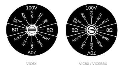
The VIC range is supplied as standard with the switch in the 100V/70V position. If you accidentally connect the system to low impedance  $8\Omega$ , it will not cause any damage to the loudspeaker but it will perform well below its performance. If you accidentally connect the loudspeaker to a 100V/70V network in the  $8\Omega$  position it will be severely damaged.
