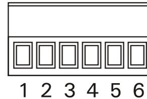
(\*\*) The WPaMIX-T / WPaMIX-TUS requires an external 24VDC power supply (connected to terminals 4 and 5, min 30mA) or 15VDC (connected to terminals 4 and 6, min 30mA). We suggest using the Ecler WP24-PSU, which can power up to twenty WPaMIX-T / WPaMIX-TUS units (depending on voltage losses caused by cable lengths and sections).
