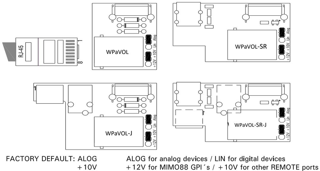
Figure 5: Internal jumpers
