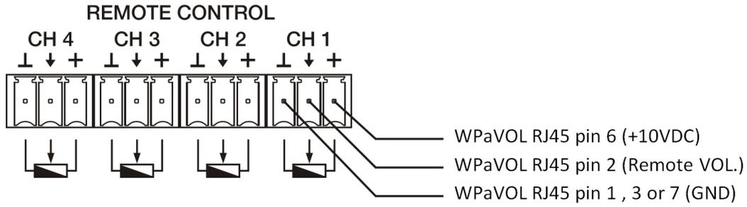
Figure 6: WPaVOL / WPaVOLUS / WPaVOL-SR / WPaVOL-SRUS connection to remote-control ports
