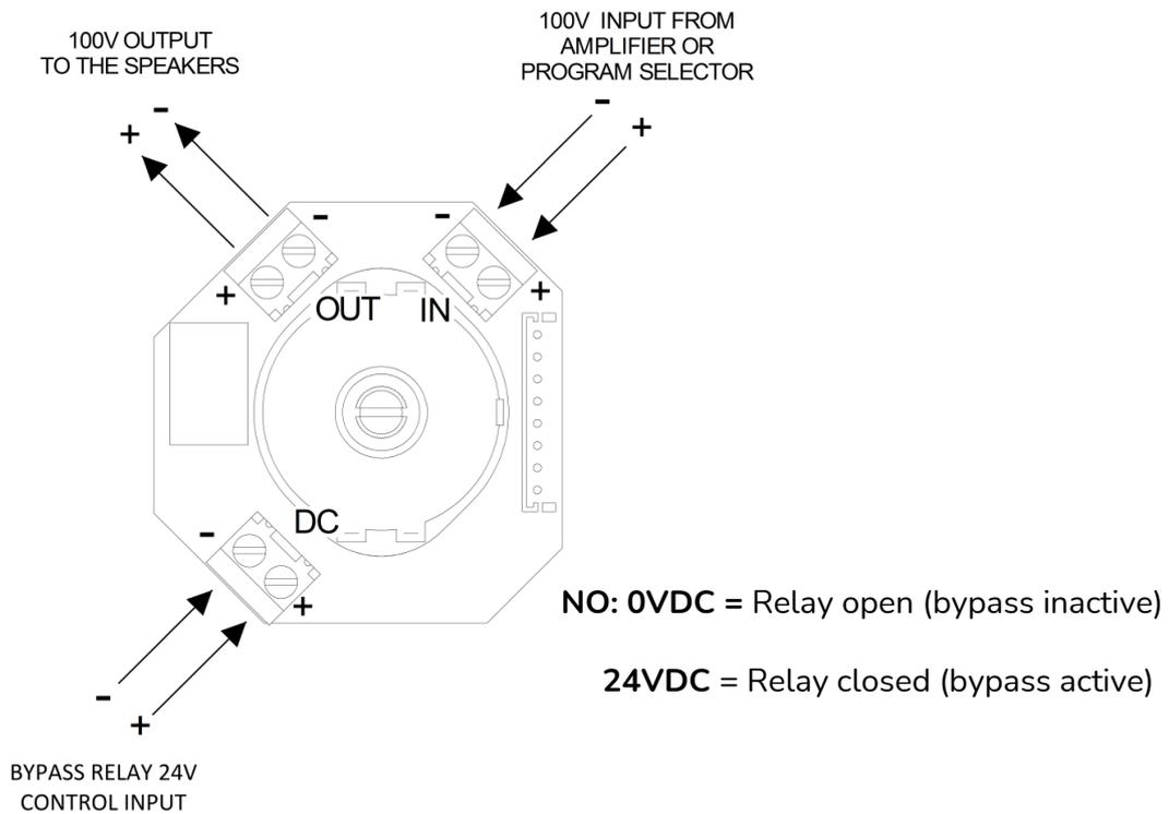
Figure 12 WPaH-AT100 connection diagram
