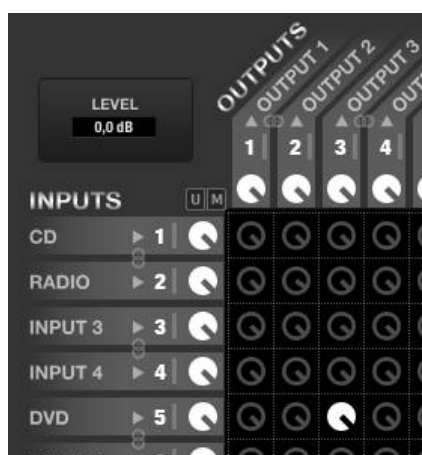
MUTE OFF for input 5 – output 3 (send enabled)
