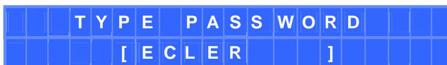
Using an encoder (ZA to ZB), edit the selected character, and using the PARAMETER key, select the next character to edit. Finally, press SHIFT + ENTER to validate the entered password.
