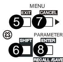
The left and right MENU keys (5, 7) allow scrolling through the different pages of the unit's setup menus.
