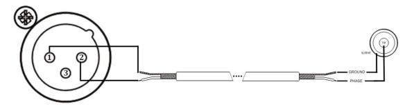
2. Connection from balanced output to unbalanced input
