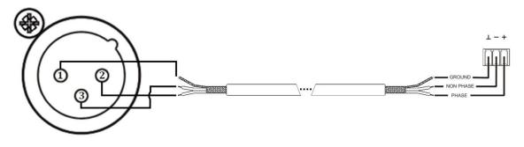
1. Connection from balanced output to balanced input
