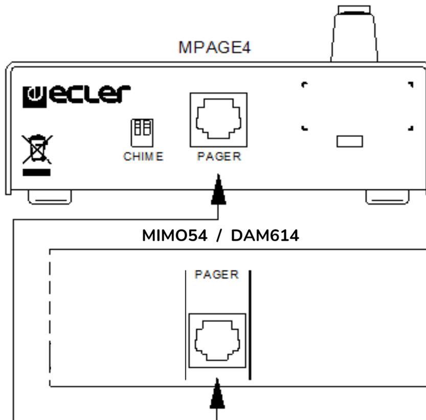
2. Activation of the carillon melody (optional). With the two CHIME (6) micro-switches on the rear panel of the MPAGE4 it is possible to: deselect the carillon melody (both set to OFF) or select one of three carillon melodies combining the ON and OFF positions (ON-OFF, OFF-ON and ON-ON). ON position = micro switch down.
