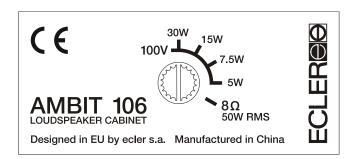
The AMBIT106 has 4 power handling levels for the 100V line. Depending on the intended use, the speaker output can be attenuated more or less. In the zones where sound intensity should be low, place the switch in the 5W or 7,5W position. If sound intensity should be high, place the switch at 15 or 30W.
