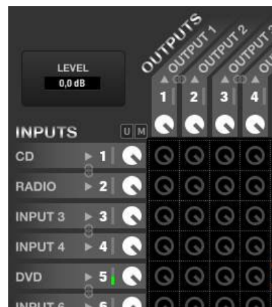
MUTE OFF for input 5 – output 3 (send enabled) MUTE ON for input 5 –output 3 (send disabled)
