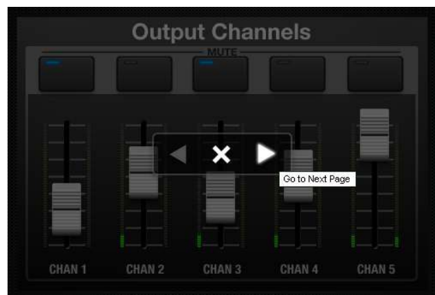
Double-clicking on a empty space of the screen shows the left and right arrow keys and the X symbol which is used to return to the root display of the available project panels (same function as the ESC key)
