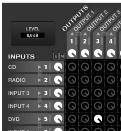
MUTE OFF for input 5 – output 3 (send enabled)
