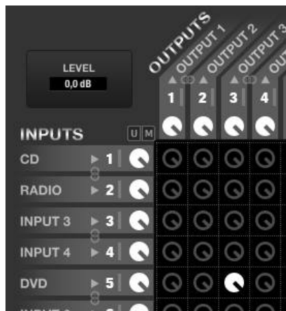
MUTE OFF for input 5 – output 3 (send enabled) MUTE ON for input 5 –output 3 (send disabled)
