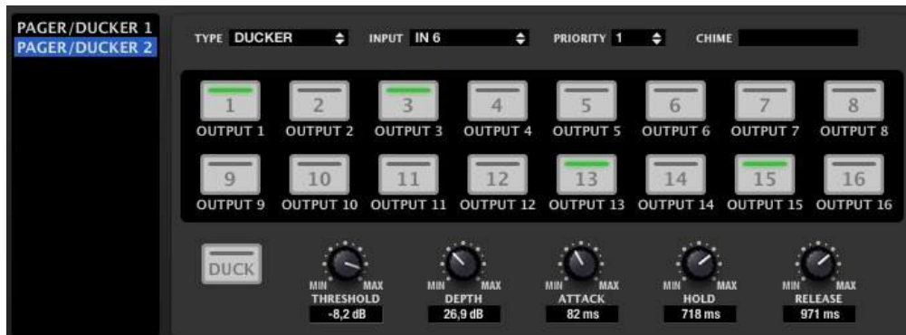
Example: module #2 configured as a DUCKER, audio input IN6 and zones 1, 3, 13 and 15 enabled for priority broadcasting of IN6 signal when it exceeds the threshold, attenuating the existing audio content in the affected outputs
