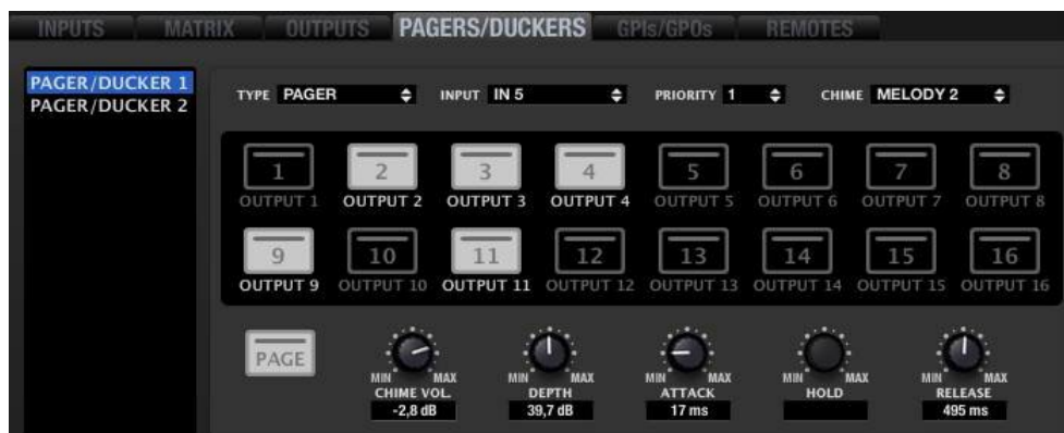
Example: module #1 configured as PAGER, audio input IN5 and zones 2, 3, 4, 9 and 11 enabled for messages sending from an eMPAGE / MPAGE16 console
