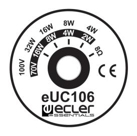
eUC106 is supplied with the switch in the 70V / 100V position. If you accidentally connect the system to a low impedance  $8\Omega$  line, it will not harm the speaker, but the speaker will perform below its real performance level. If the speaker is in the  $8\Omega$  position and is accidentally connected to a 70V / 100V line, it will be seriously damaged.
