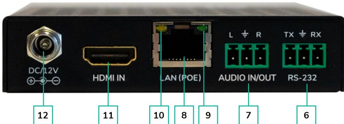
**6. RS-232:** Serial port for remote control. Signal pass-through supported.
