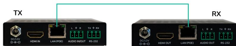
1. Connect the source device to the VEO-XTI1CG2 transmitter to the HDMI® port.
