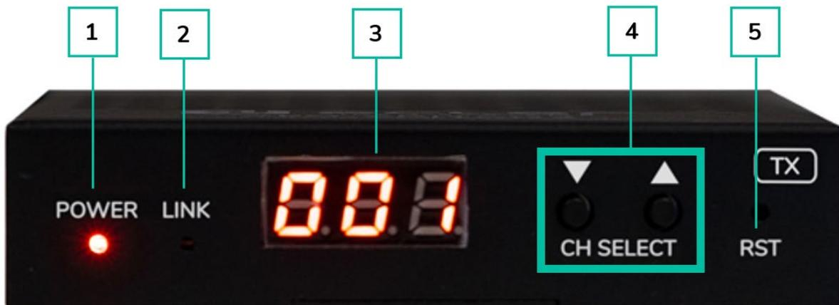
1. **POWER LED:** The LED flashes when the device is power supplied and stays lid (RED) after the start up is complete.
