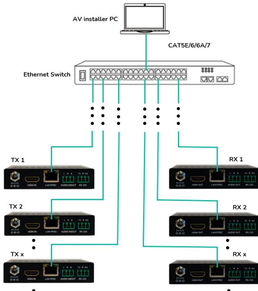
1. **Set the IP address** for each transmitter and receiver.
