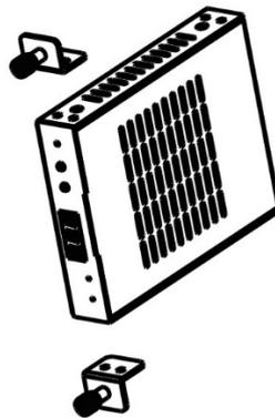
2. Insert the product with mounting ears into a 3U rack (up to 12 units can be installed vertically), as shown in the figure below:
