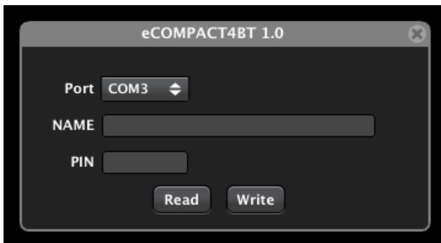
5. Select the correct COM Port and click on READ button. Verify that the information about NAME and PIN of the device appear on the screen. This information must be like the following (factory defaults):
