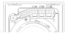
**Note:** If the system is accidentally connected at low impedance  $8\Omega$ , this will not cause any damage to the loudspeaker, but it will reduce its performance considerably below its capabilities.
