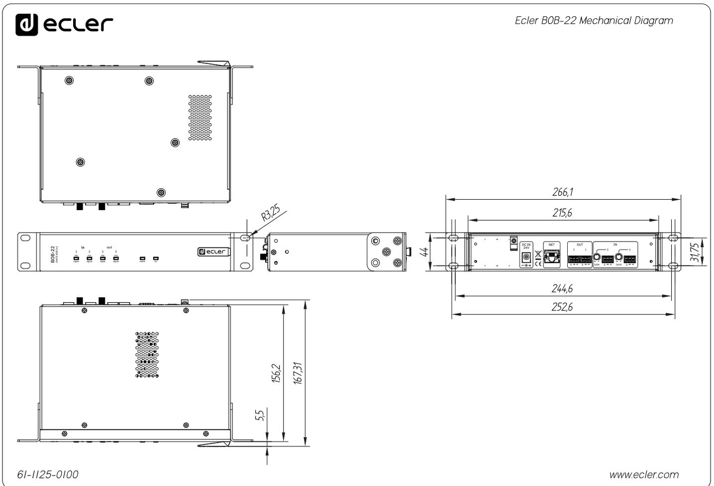
All the measurements are in mm
