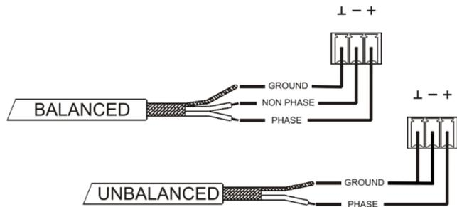
**⚠** For unbalanced connection short-circuit pin ⊥ to pin - as reported on the picture.
