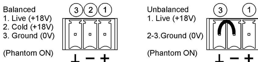
**!** Microphones must be low impedance (200 to 600 Ω) and monophonic.
