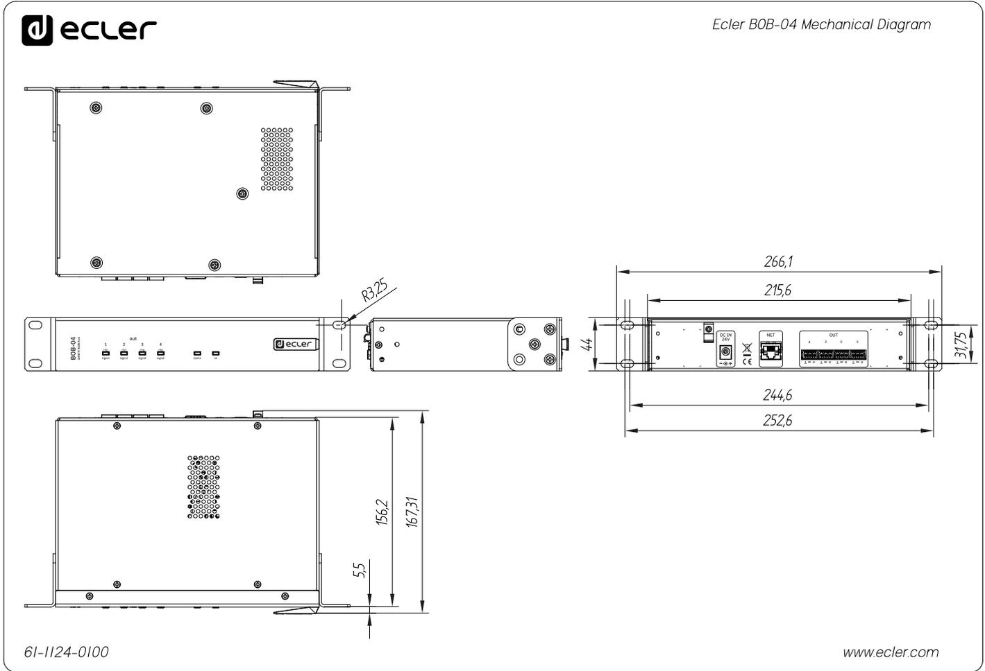
All the measurements are in mm
