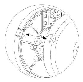
9. Align the speaker to the desired position on the vertical and horizontal axes
