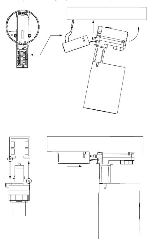
Connection to a rail GLOBAL Trac Pro (three-wire lighting anchorage system)
