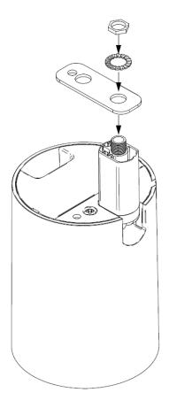
**4.** Make the connections, taking into account the colour coding for high and low impedance explained in point 3 of the instructions for installation on the lighting rail. If desired, use the screwable rail on the base of the surface mount. Attach the speaker to the threaded bar or truss and orient the speaker to the desired position along the vertical and horizontal axes
