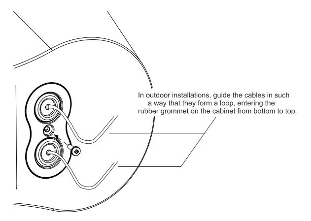
In outdoor installations, use a round tool to drill the grommets.
