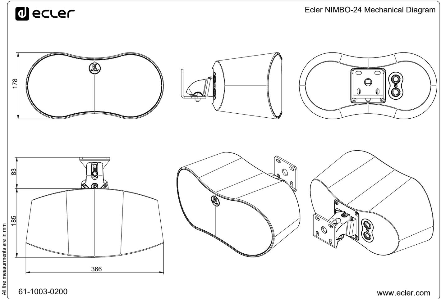
All the measurements are in mm
