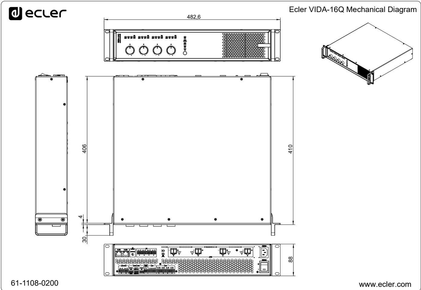
All the measurements are in mm
