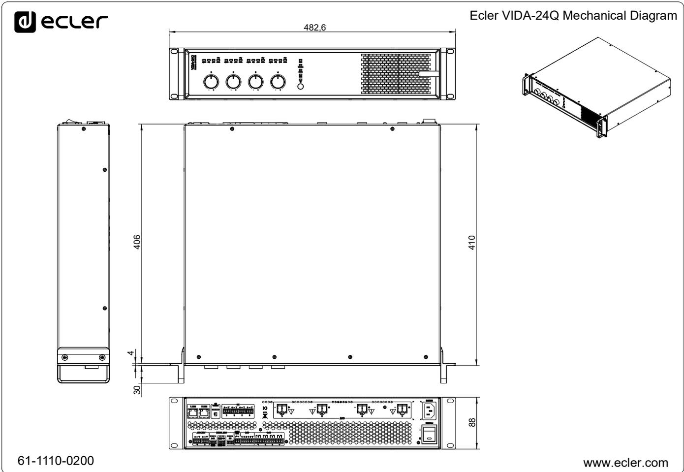
All the measurements are in mm
