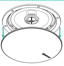
Gently pull the frameless magnetic protective grille to remove it from the loudspeaker.
