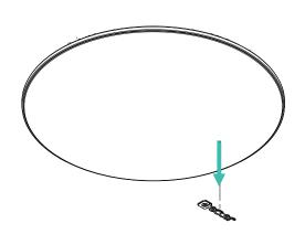
The Ecler logo has an adhesive strip that allows it to be easily removed and reattached. Remove the Ecler logo by simply pulling it off the grille.
