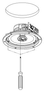
Place the speaker in the newly cut hole. Hold it in position with your hand and insert it carefully, ensuring that the three rotating fasteners are retracted.
