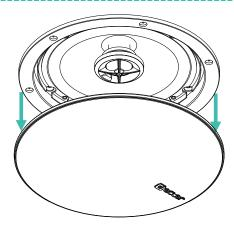
Gently pull the frameless magnetic protective grille to remove it from the loudspeaker.
