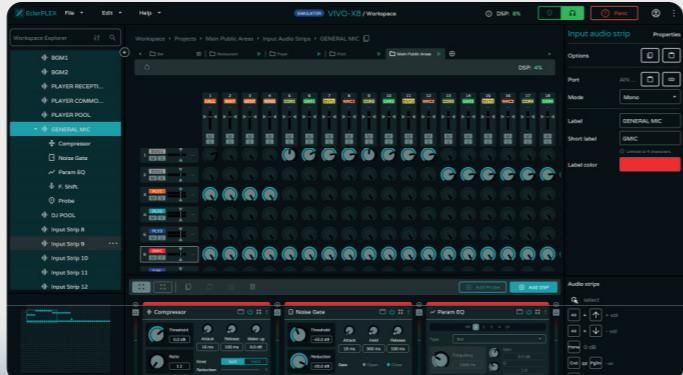
It allows users to also customize audio I/O strips in a modular way, using individual audio DSP blocks in a sequential arrangement. Several projects can be run simultaneously, up to the maximum I/O global and DSP capabilities of the HW Host unit in use. The Host unit is able to use Guest units' resources in its projects through a regular LAN, creating a mesh of EclerPLEX devices.
